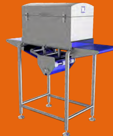
The conveyor belt used in fish processing with the "vision robot" that performs the measurements and collects data.
